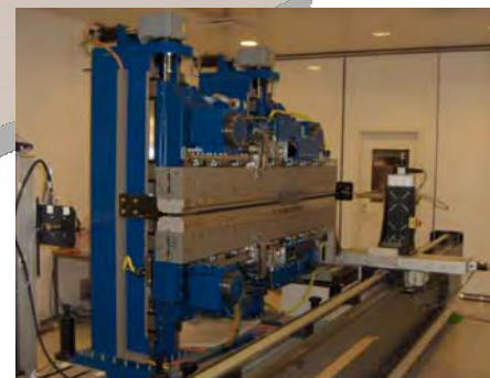
The EPU undergoing magnetic testing in Denmark at Danfysik A/S
