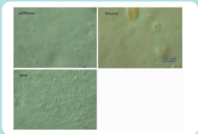
Surface appearance of zinc oxide paint samples formulated with different oils and aluminium stearate.
