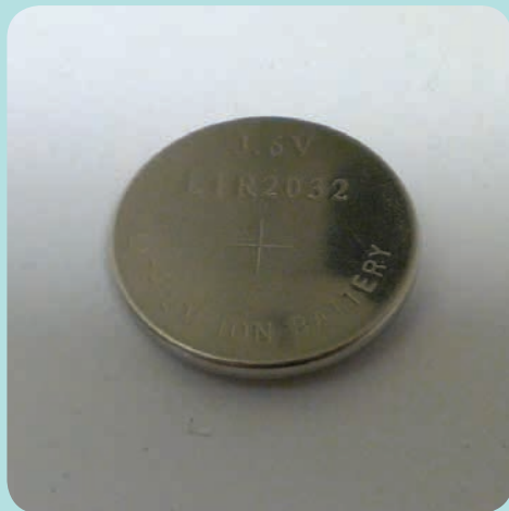
(L) Typical research scale coin cells used to test the electrochemical performance of these batteries. (R) The model of the major compound \text{Li}_4\text{Ti}_5\text{O}_{12-x}\text{Br}_x (black line) fitted to synchrotron x-ray diffraction data (red crosses). The arrows and inset indicate the presence of extra un-matched reflections which illustrate that there are other compounds in this electrode material.
