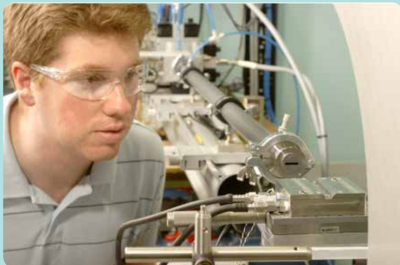
Dr Nathan Webster setting-up a sample stage for in situ studies on the PD beamline.
